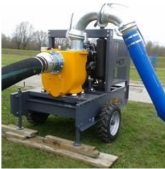
Pump unit on a mobile frame
